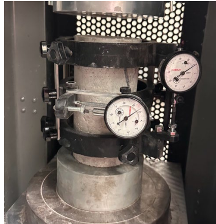
Figure 3.24 Test setup for Static Modulus of Elasticity.
