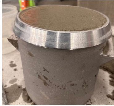
Figure 3.17 Unit weight measurement.
