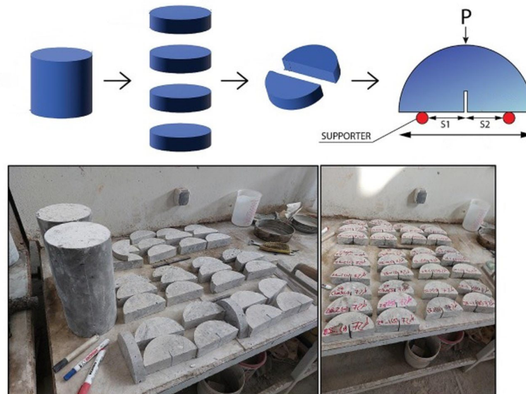
Figure 2.5 Steps for SCB specimen preparation (Ghodratnama et al., 2025).
