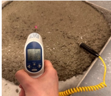
Figure 3.15 Fresh concrete temperature measurement.
