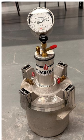
Figure 3.18 Air pressure measurement (meter type-B).
