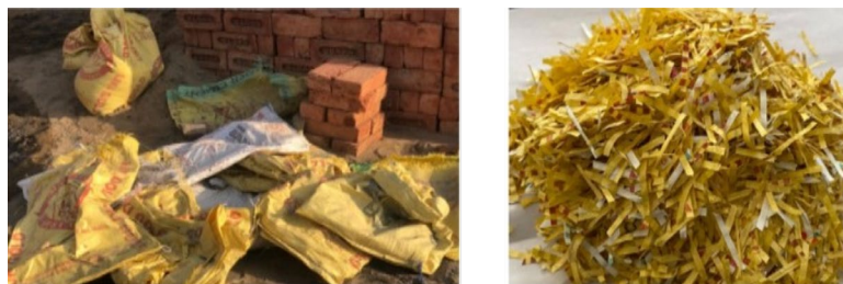
Figure 2.4 a) PP plastic bags at the construction site, b) PP fibers after shredding (Rafiq Bhat et al., 2023).
