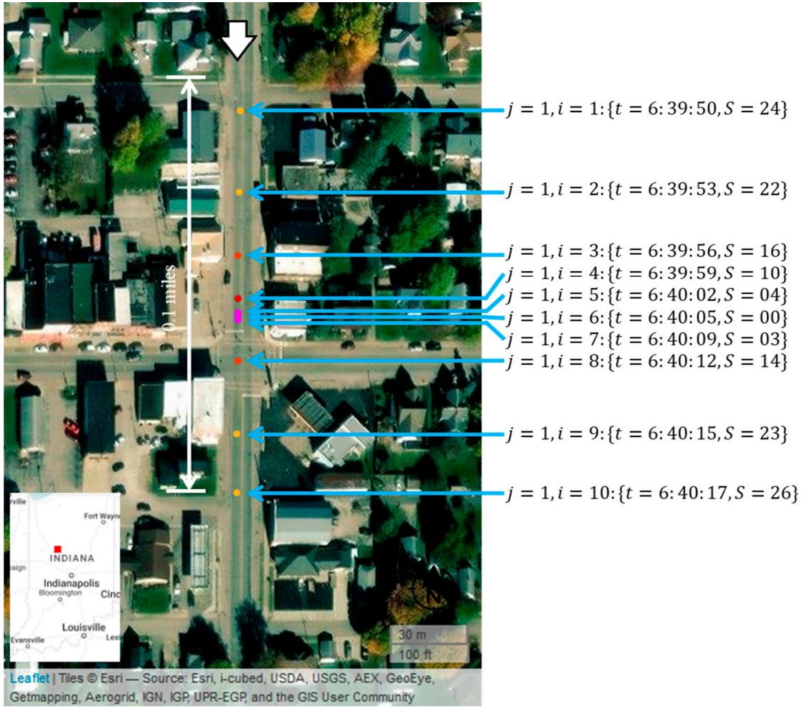
Speed (mph): ■ 0 to 5 ■ 5 to 10 ■ 10 to 20 ■ 20 to 30 ■ 30 to 40 ■ 40 to 50 ■ > 50 Figure 5.2 A Sample of One CV Trajectory/Journey Through a Segment With Ten Waypoints.
