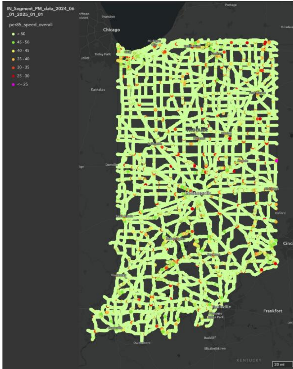
Figure B.2 2024 Annual Segment PMs – 85 th Percentile Overall Speeds Color Coded by Speed Bins. https://purdueuniversity.maps.arcgis.com/apps/instant/sidebar/index.html?appid=f23cb7e13a774925acee2c5b0b5c3dee
