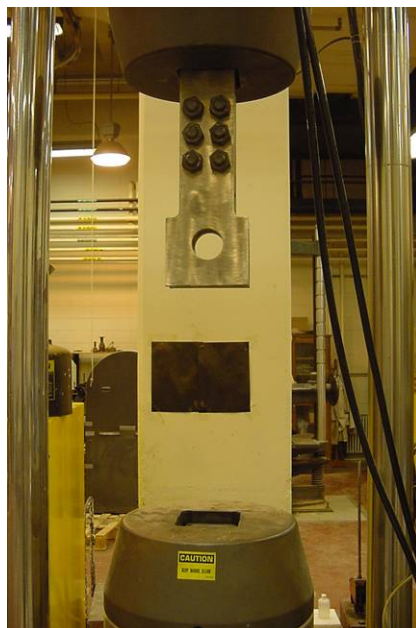
Figure C.21 Photograph of Attachment Utilized in Testing Eyebar End Connections in the 220-kip MTS Servo-Hydraulic Testing Machine
