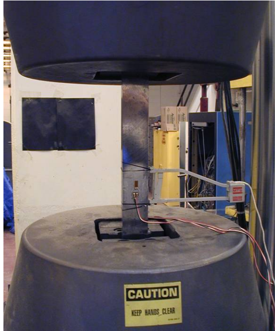
Figure C.15 Tensile Coupon from Bell Ford Bridge in Grips of MTS Testing Machine before Testing
