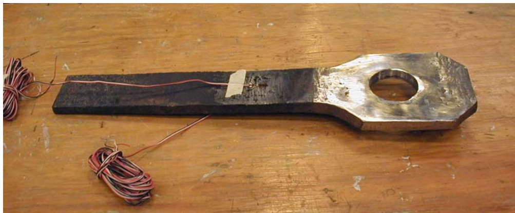
Figure 3.34 Eyebar B Before Testing and After Surface Ground and Strain Gages had been Attached
