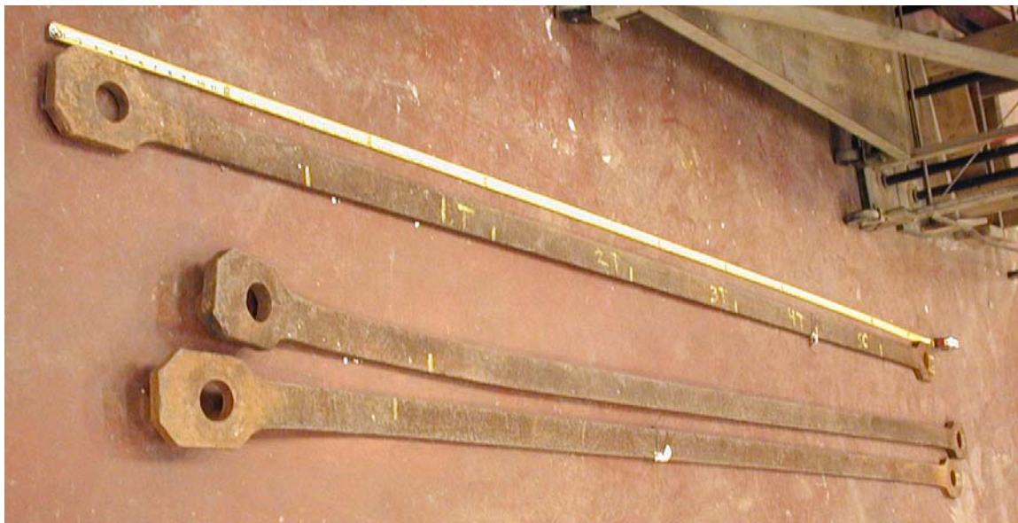
Figure 3.3 Donated Eyebars 4 and 5 Along With a Similar Eyebar that Was Straightened and Used in the Reconstruction of the Bell Ford Bridge
