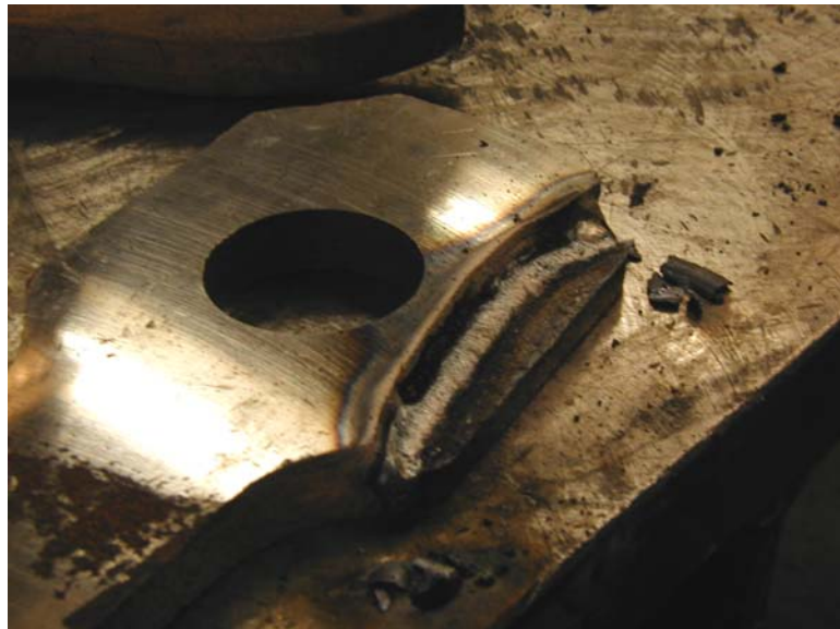
Figure D.8 Initial Pass Pattern on Eyebars A
