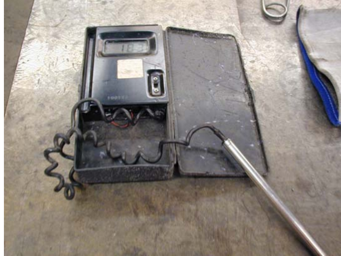
Figure C.5 Pyrometer Used to Determine Temperature of “Red Hot” Wrought Iron.
