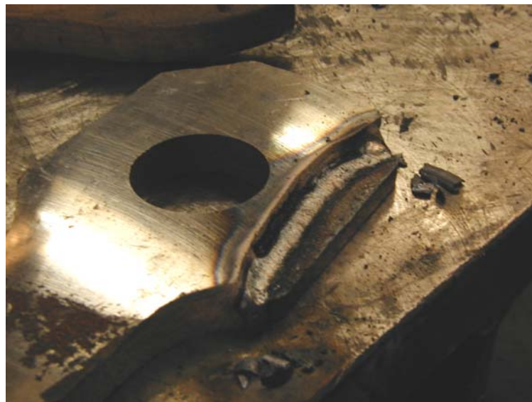
Figure 3.25 Eyebar Connection A After Material Was Removed to Simulate Corrosion
