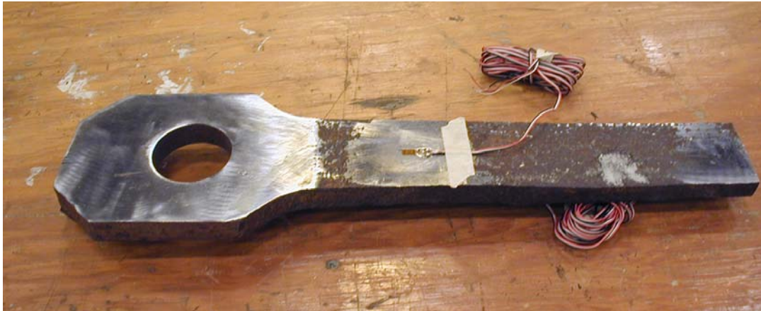
Figure 3.33 Eyebar A Before Testing and After Surface Ground and Strain Gages had been Attached
