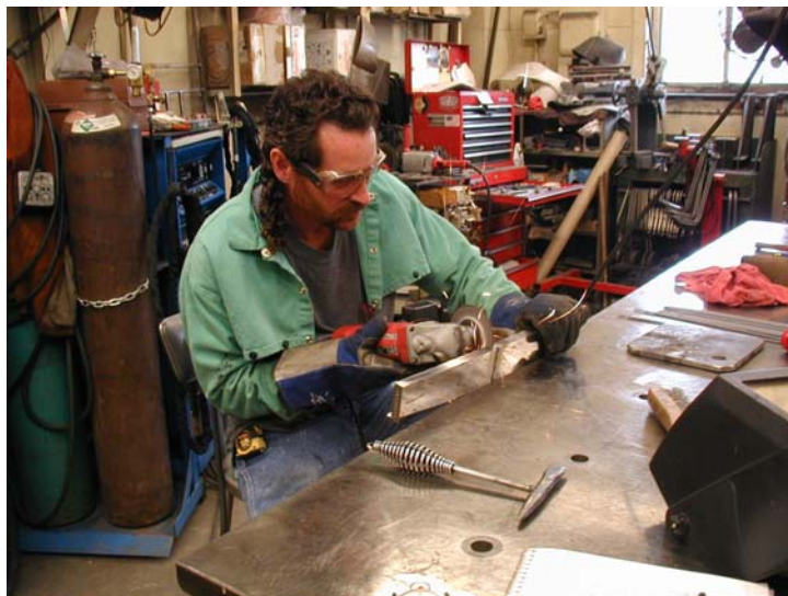
Figure C.9 Back-grinding of Initial Root Pass before Second Weld Pass is Placed
