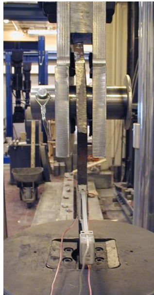
Figure 3.36 View of Eyebar B in Testing Machine with Extensometer Attached Showing Slight Amount of Distortion in Eyebar
