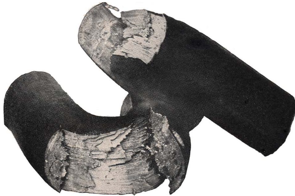
Figure 2.1 Fracture Showing Fibrous Nature of Wrought Iron. (Aston, 1949)
