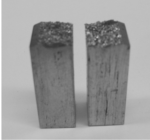
Figure 4.21 Cleavage Fracture of Charpy Impact Specimen (LU, LS Type)
