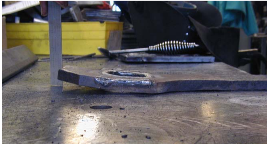
Figure D.9 Resulting Heat Distortion From Welding in Eyebar B
