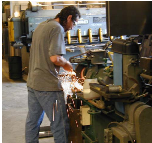
Figure C.6 Rotary Grinder used to form Double V Butt Joint in Welded Specimens
