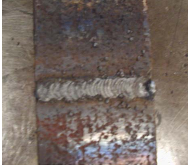
Figure D.5 Completed Weld Before Surface Grinding
