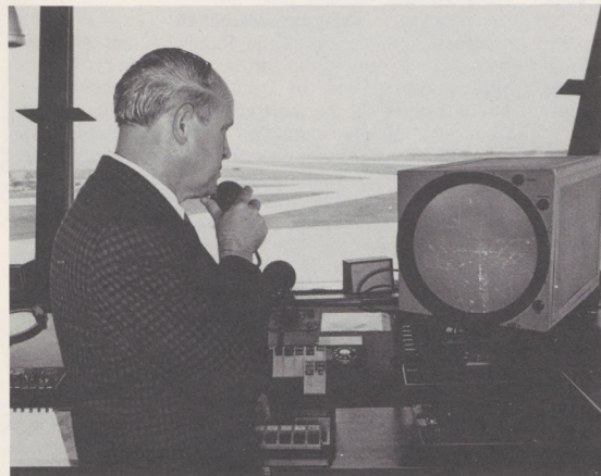
Donald Weaver, a supervisor in the control tower at St. Petersburg-Clearwater Airport, looks at a BRITE-2 display, relayed to the tower cab via microwave equipment from the search radar at Tampa International Airport, 11 miles distant.
