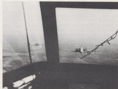
Flying in formation, two glider-towing C-47s are seen from the glider pilot's seat, with the vital tow line seen in the right of the picture.
