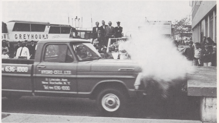
A dramatic demonstration shows how water-filled plastic cells attached to bridges or abutments can soften collision impacts to such a degree that driver and passengers can walk away smiling and uninjured. The plastic cells for highway bulwarks were rammed at 30 miles per hour without hurting the driver.
