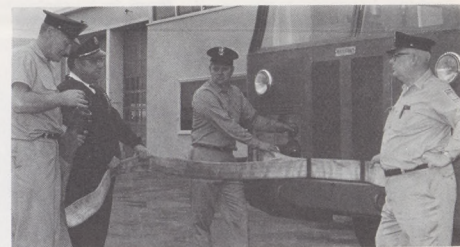
No item of equipment is too small to escape a regular check and inspection by FAA firefighters. At DCA, Otto Evans inserts a gasket in a soft suction hose carried by the facility's Ward LaFrance 750 gallons-per-minute pumper. Assisting are (left to right, after Evans): Capt. William L. Walker and Firefighters Robert Brown and Archie H. Layton.
