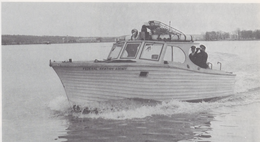
From the south end of DCA, the 32-foot FAA rescue launch (at one time a Cuban gun runner) can make 30 knots if necessary to reach a downed aircraft or a boat in jeopardy (sailboats must be kept out of areas near approach paths). Crew for training exercise consisted of Capt. William L. Walker, Training Officer, Lt. William Wynne and Firefighters Robert K. Brown and Jack Dant. Two 17-foot launches are kept at north end of Washington National.
