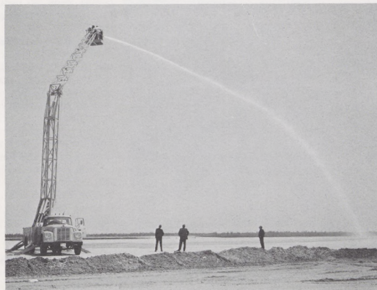
NAFEC firemen at the top of the 70-foot high aerial tower truck use a hose line in a practice session. The truck, which has outriggers to prevent tipping, is also used by workman for access into high places.
