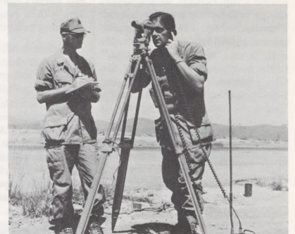
Tracking flight-check aircraft on GCA approach, FAAer John Reynolds verifies accuracy of glide-slope settings at the Kontum Airfield in South Vietnam while SFC John Myers records data.
