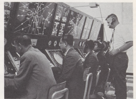
Back-lighted sector panels, radar and rapid radio communications which expedite training of today's air traffic controllers (above), are in sharp contrast to the handwritten flight strips and relatively unsophisticated teaching aids in vogue a quarter of a century ago (below).
