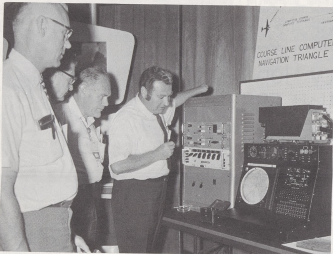
Bernhart Dinerman (right), shows pilots how a course line computer is used in navigation.
