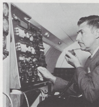
New lightweight inspection console, being checked out by Leo Sutter of the National Field Inspection Division in Oklahoma City, is designed especially for the Sabreliner. Weighing only 300 pounds—one fifth the weight of the pre-solid-state console—the unit receives as many incoming signals from ground nav aids as do consoles in the much larger Convaers.
