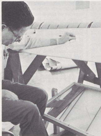
Fabrics for ailerons, rudders, elevators and other airfoil sections of aircraft must be sewn properly before the section is dope-covered. Here, Shedrick Rutledge has rigged a mirror to reflect under the wing so he can see to bring his long needle back through the fabric.
