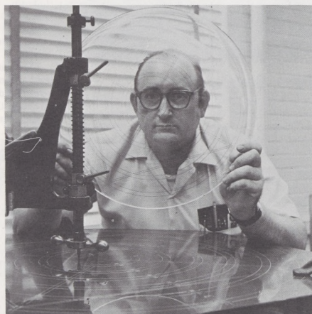
Clear plastic, pantographed to show aircraft "blip" positions on a radarscope, is inspected by Charles Lattimore. With this plastic cover, a controller can pinpoint a plane's location.
