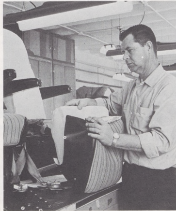
Aircraft Services Base upholsterer Johnny Holloway prepares an FAA Lockheed JetStar seat for new upholstery.
