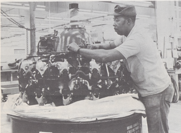
Engine mechanic Vernon McCaslin works within the engine nacelle from a Convair before moving the overhauled turbo-prop engine into the nacelle for positioning and bolting. Below, an engine for one of the agency's "Gooneybirds" is unpacked by ASB mechanic Joseph B. Neal, Jr. (In maintenance parlance, it's really an R-1830-94 engine, for a DC-3.)
