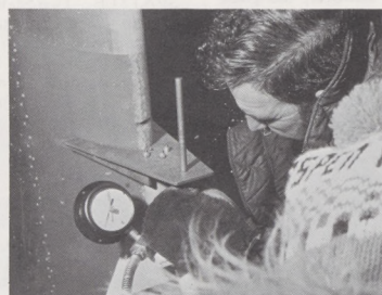
Donald Millar, project manager, NAFEC, checks adhesive characteristics of one of the products being tested by the FAA. He is shown using a special jig designed at NAFEC especially for these tests. (Below): Icing research tunnel controls are worked by Harry Minster (seated), NASA aerospace mechanic. Millar checks console for proper icing conditions and air velocity.
