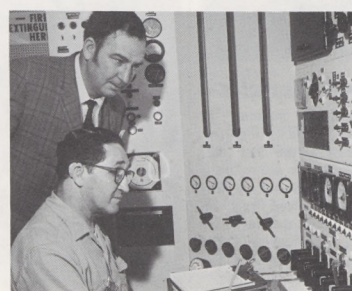
Donald Millar, project manager, NAFEC, checks adhesive characteristics of one of the products being tested by the FAA. He is shown using a special jig designed at NAFEC especially for these tests. (Below): Icing research tunnel controls are worked by Harry Minster (seated), NASA aerospace mechanic. Millar checks console for proper icing conditions and air velocity.
