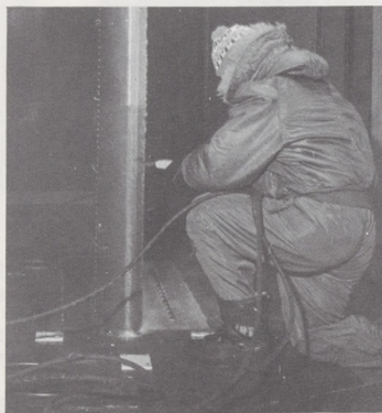
Clad in Arctic clothing, NAFEC technician James H. Dailey prepares the leading edge for adhesion test. Here he uses an electric divider to make room for the special jig which tests the amount of pressure needed to remove ice from the wing.
