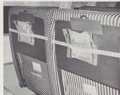
Hoods weigh three ounces and are very compact when folded. For recent FAA evacuation tests, hoods were attached to the underside of passenger seat trays, providing quick availability.
