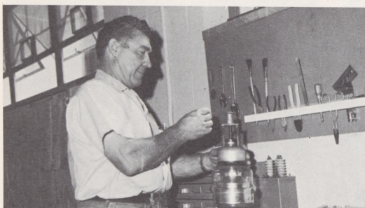
Repairing a vacuum condenser, Engelbach uses a repair kit jig of his own design. The kit was submitted as part of the Employee Suggestion program and is expected to be adopted for agency-wide use.
