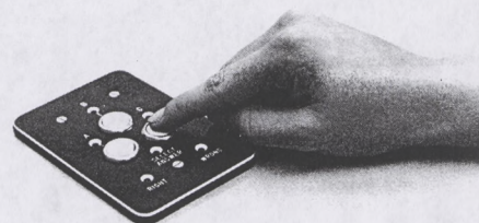
Students' grasp of the subject just presented can be seen quickly by the instructor, after each student selects his "a, b or c" answer and results of the entire class show up on a master console panel. Several incorrect responses indicate the instructor should review points needing clarification.
