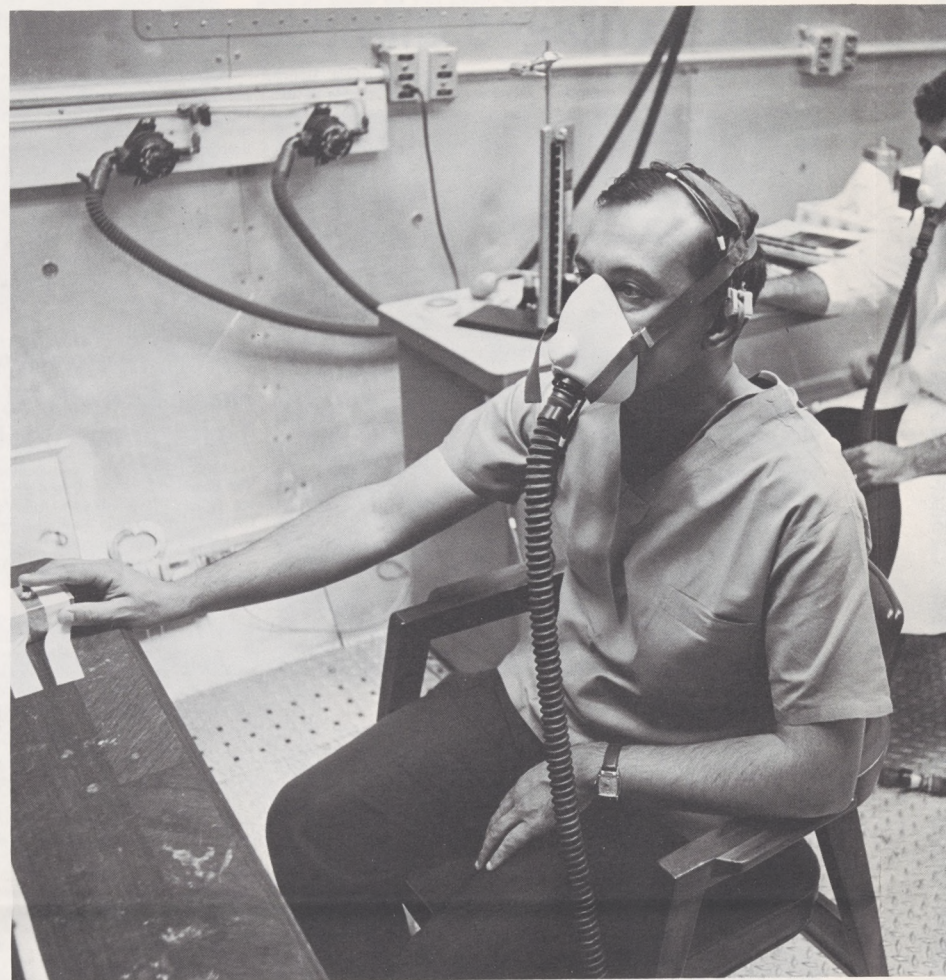
In the Psychology Laboratory, Robert Lewis operates research equipment which permits a variety of tasks to be required of the operator under various conditions of workload. Tasks include visual and auditory monitoring, signal detection, pattern identification, mental calculations, reaction time and team problem-solving. For team problems, four additional operators participate. The same psychomotor functions are used in piloting aircraft. It is hoped to establish correlations between laboratory tests and real-life flight circumstance.
