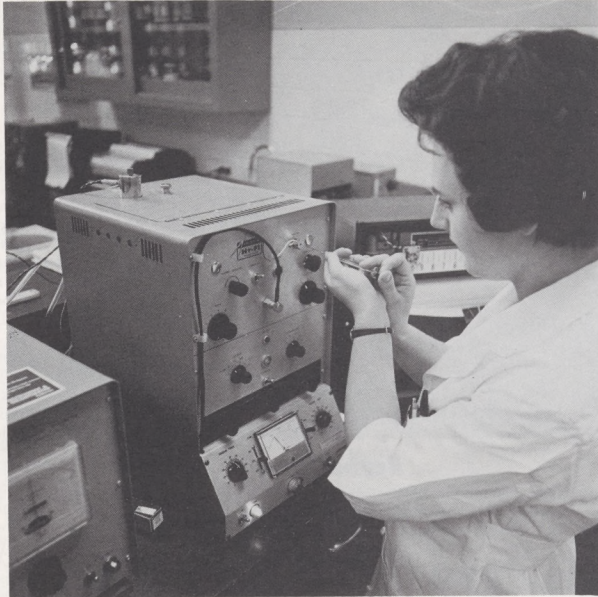
To measure alcohol content, Mrs. Pat Roberts injects blood sample from an aircraft accident victim into a gas chromatograph.
