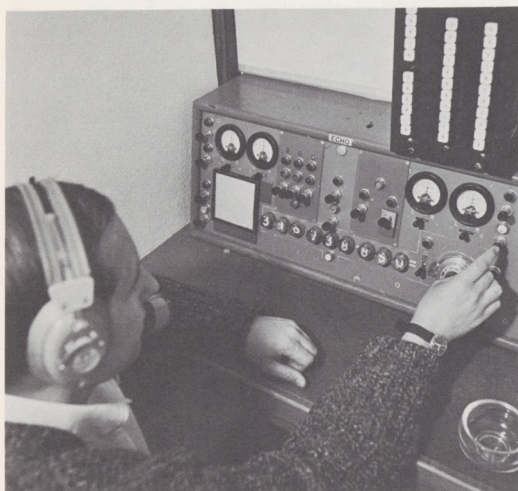
In the Psychology Laboratory, Robert Lewis operates research equipment which permits a variety of tasks to be required of the operator under various conditions of workload. Tasks include visual and auditory monitoring, signal detection, pattern identification, mental calculations, reaction time and team problem-solving. For team problems, four additional operators participate. The same psychomotor functions are used in piloting aircraft. It is hoped to establish correlations between laboratory tests and real-life flight circumstance.
