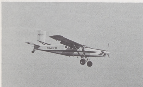
Relief from burgeoning traffic's demands on existing airports may come from separate STOL ports. Using them, aircraft such as the Fairchild-Hiller "Heli-Porter" (shown above) can land or take off in a few hundred feet. Tests at NAFEC near Atlantic City will determine just how short such runways can be.
