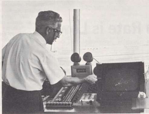
Television has extended the eyesight of controllers at the local position in the tower cab. Here Donald Capellas watches a TV monitor that is especially helpful at night, when visual acuity is greatly diminished and to determine spacing for landings on Runways 4 and 8.
