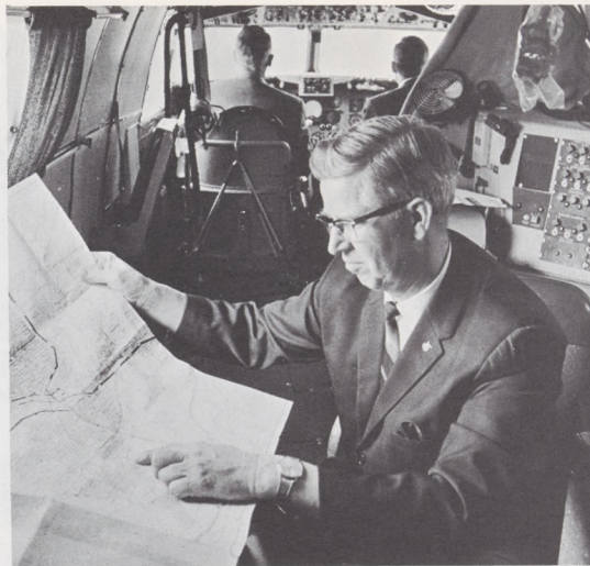
Chief Tom W. Smith (left) and Frank Wallis, of the Battle Creek, Mich., FIDO, pilot an FAA electronically-equipped DC-3 while FCC Engineer Edward Atems (foreground) checks a map to determine the location and source of radio interference encountered between military aircraft and local ground stations in the Battle Creek area.
