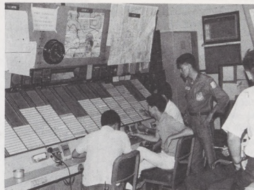
Vietnamese personnel control Northern Sector traffic in the Saigon Center. Flight data strips represent location of individual aircraft, with each strip giving origin, destination, altitude, speed, flight number and ETA at next checkpoint.
