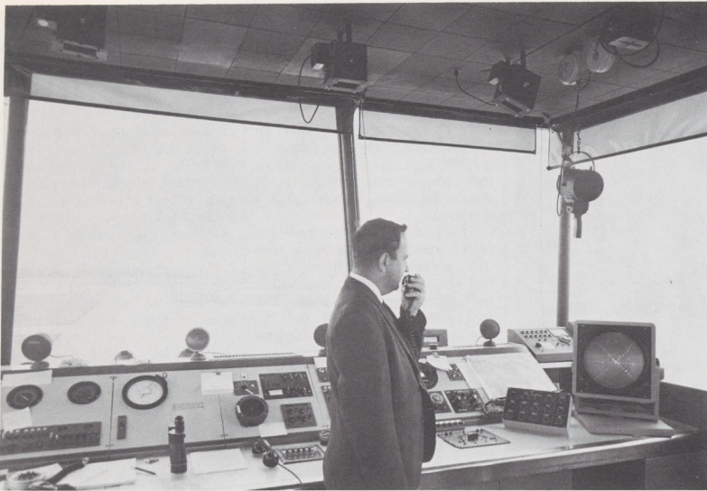
This new bright display can be read in the changing bright lights of a control tower cab thanks to a new technique of epoxy bonding a filter to the front face of the glass plate TV tube. The new tube has an extremely high light-level output capability.
