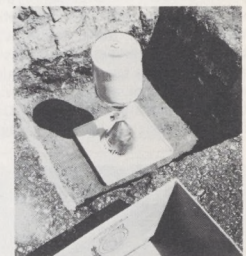
A density sand cone measures the volume of soil removed from the test hole. Other tests done in a mobile laboratory determine asphalt content, gradation, maximum density, soil plasticity, etc. of an airport.
