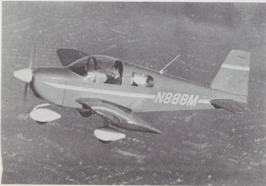
▲ Pioneering new structural construction techniques, American Aviation Corporation's "Yankee" cruises at 137 m.p.h. and has a range of 378 nautical miles. The fuselage is not riveted, but of honeycomb panels bonded at 250-285 degrees. Dick Kemper, general manager of operations, is the pilot.
