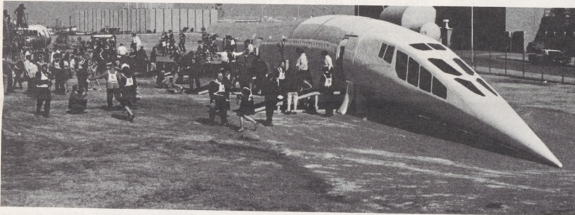
Passengers immediately after the first evacuation test of a model SST at the agency's Aeronautical Center, Oklahoma City. Two hundred eighty-nine were evacuated in one minute, 27 seconds from seven exits. Four double-doors on other side of aircraft mockup were used in subsequent testing.
