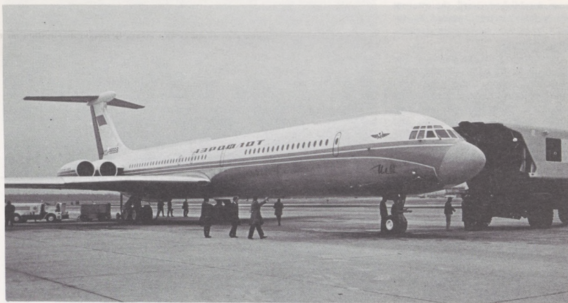
▲ The IL-62 is roughly equivalent in size and performance to the Boeing 707 and DC-8. Note how it is capable of mating with Dulles' Mobile Lounge.
