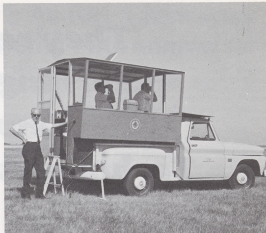
Arch R. Moody, of airway facilities at Oklahoma City, stands by the portable tower cab he designed and built for use in the area to handle air traffic attending fly-ins, air shows, and Oklahoma University's home football games.
