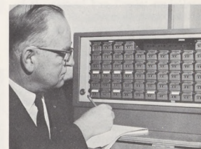
New telephone equipment like this being used by Joseph Greten will improve FSS service by guaranteeing "first come, first served" answering to callers. This is a prototype now being used at Washington National Airport.
