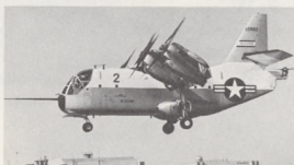
... it makes a short takeoff with wing at a 35-degree angle.
