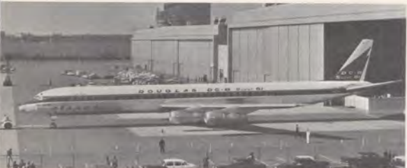
Douglas DC-8 Super 51, largest existing jet airliner, carries 251 passengers, measures 187.4 feet in length.
