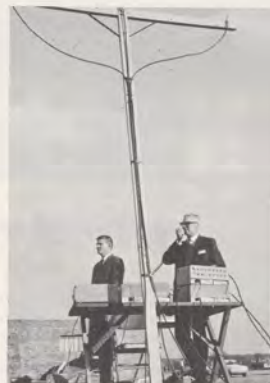
COLLAPSIBLE TOWER — Jerry E. Graves, Springfield, Mo., designed a collapsible antenna support for temporary towers. From left: Bob Schuerer and Richard Williams.
