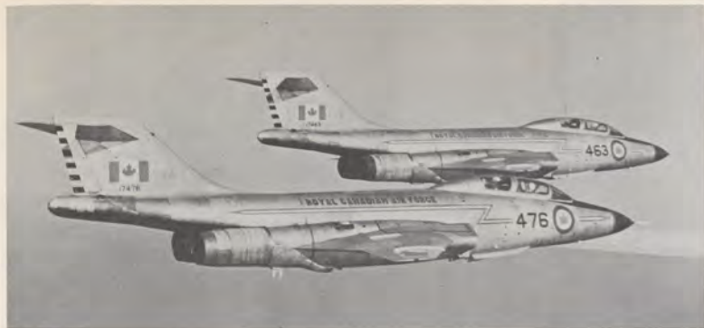
These Royal Canadian Air Force CF-101B Voodoos can speed to intercept hostile targets at 1,200 mph.
