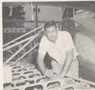
Right: Gil Carlson, pads the wings of his Aeronca Champion with styrofoam to help keep it afloat in case of an inadvertent water landing.
