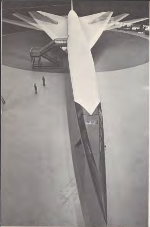
Boeing full-scale mock-up seems to 'spread its tailfeathers' as the variable sweep wing is demonstrated in triple-exposure.
