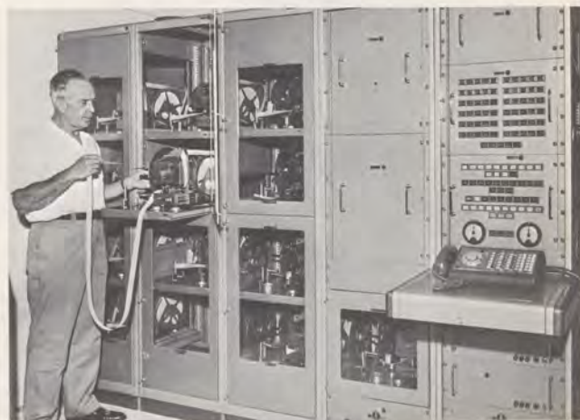
High-speed paper tape punch records weather readings.
