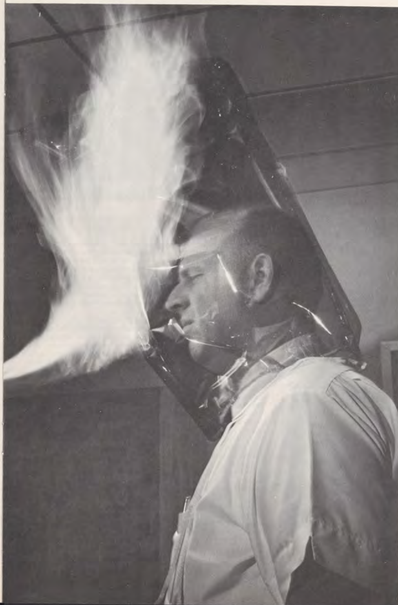
Human factors specialist Ernest McFadden demonstrates a plastic bag which may provide protection to passengers in aircraft crashes.
