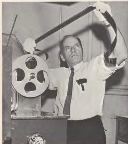
Photographer Nelson Amey takes a look at a strip of 35 mm film as it comes out of the automatic film processing machine.
