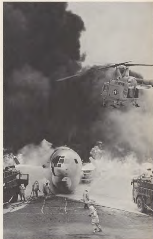
A battery of NAFEC photographers recorded a series of fire tests which studied the effects of various fire fighting equipment on the extinguishing of a burning surplus C-97 aircraft.
