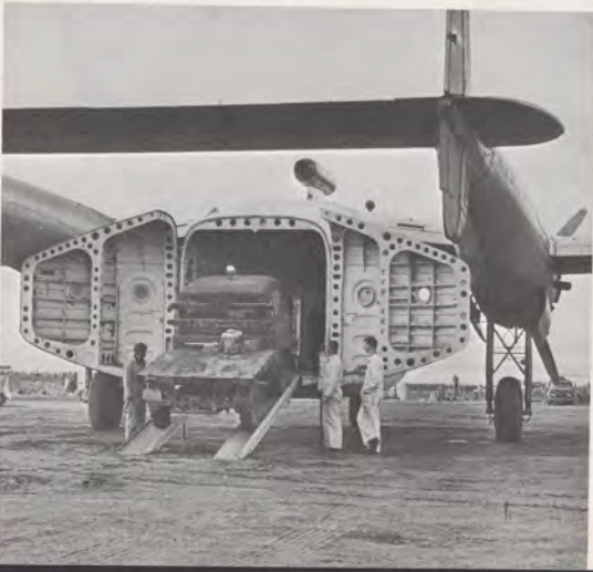
An Interior Airways C-82 at Fairbanks is one of the many aircraft used for hauling "out sized" cargo.
