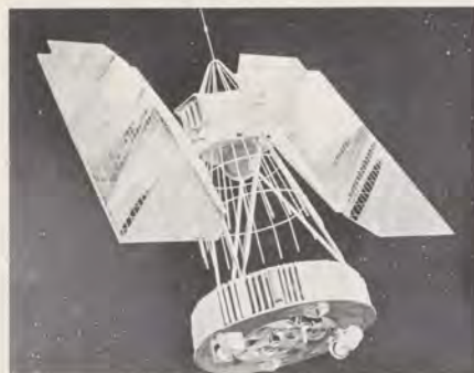
Nimbus II can obtain temperature data at various levels.
