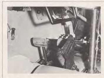
Above, the first flying couple in the Little People of America are from Richardson, Tex. Below, their plane, modified by a Dallas mechanic. It has extended rudder pedals and other redesigned controls.
