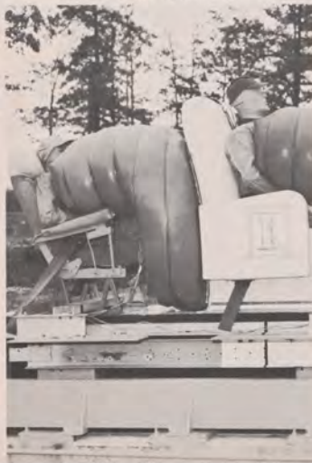
Dummies go for 75 mph ride in air bag restraint test; track ruler markings show stopping distances.
