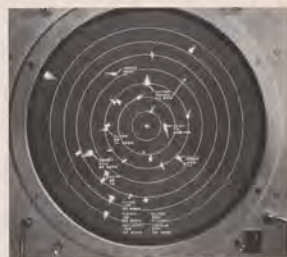
This retouched photograph of an ARTS radar scope shows electronic tags which take the place of manually controlled plastic "shrimboats" which carry less data.
