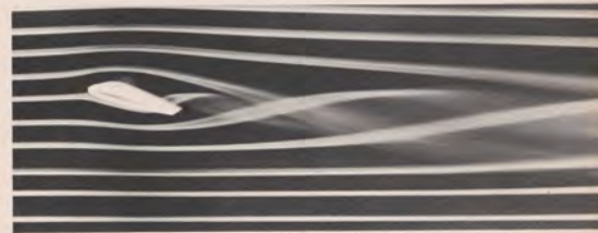
▼ Smoke flow around airfoil shows wake turbulence dangers.
