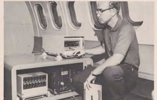
A new inflight data recorder was installed in the Agency's Convair 880 during modifications at the General Dynamics plant in California. Charles D. Sjulín, of the Aeronautical Center's Avionics Systems Engineering Branch, Aircraft Services Base, checks the recorder. The recorder will provide accurate, comprehensive reports of the functional condition of the aircraft's various systems.
