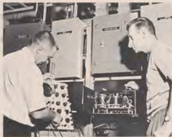
Left: Clare Krech troubleshoots electronic circuit board. Below: He and Earl O. Larsen test trigger generator for synchronizing the radar system.
