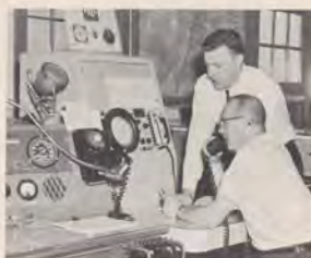
Air traffic control specialists Harry Jenkins (seated) and Ignace Ban, at console of Doppler DF installed in Kenai FSS last year. Doppler was used to aid pilot, an Air Force C-123 finally shepherded Davis to safety.
