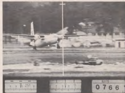
Below: Even if cross-hairs of theodolite sight are not precisely aligned on the predetermined bulls-eye of the target, data processing operators can make corrections using movable cross-hairs which compensate for the error. The theodolite facilities at NAFEC are available to industry on a rental basis.
