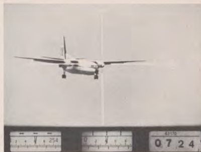
Above: A Fairchild Hiller F-27 shoots an approach to NAFEC. Theodolite is zeroed in on one engine of the plane. The scale at the lower left of the photo gives azimuth; elevation is indicated in the center scale; photo number is to right. Below: Aircraft position at moment of touchdown is recorded.
