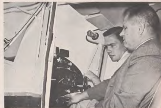
Above: General Aviation Operations Inspector Douglas B. Moore (dark suit) and Ken Nesbitt, Atlanta flight instructor, run check list before takeoff. Below: Moore watches as Nesbitt checks aircraft oil level. Inspectors in the traveling show stress the importance of detailed preflight inspections using printed check list.
