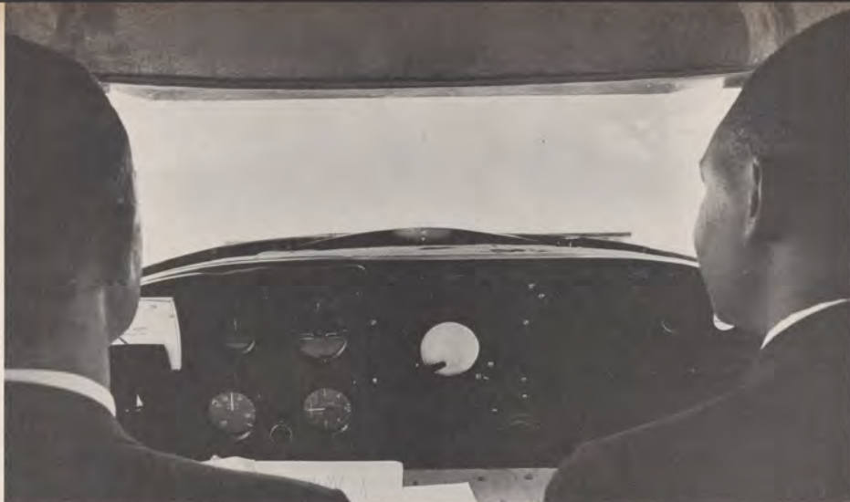
Inside "cockpit" preparing for a simulated approach in the fog chamber where scientists are studying the configuration and intensity of airport lights.
