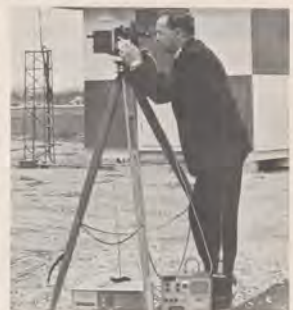
Richard W. Ladzinske adjusts the electronic theodolite which he invented and which won him recognition.
