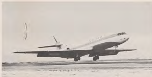
The automatic landing system gently lands a Caravelle jetliner without the need for pilots to touch any controls.
