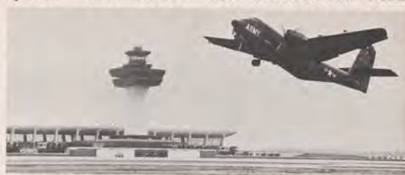
A VC-28 Caribou, on loan from the Army, is pulled off the Dulles helipad after a takeoff run of less than 500 feet in V/STOL tests being conducted by the Agency's Aircraft Development Service. The landing roll is even shorter.
