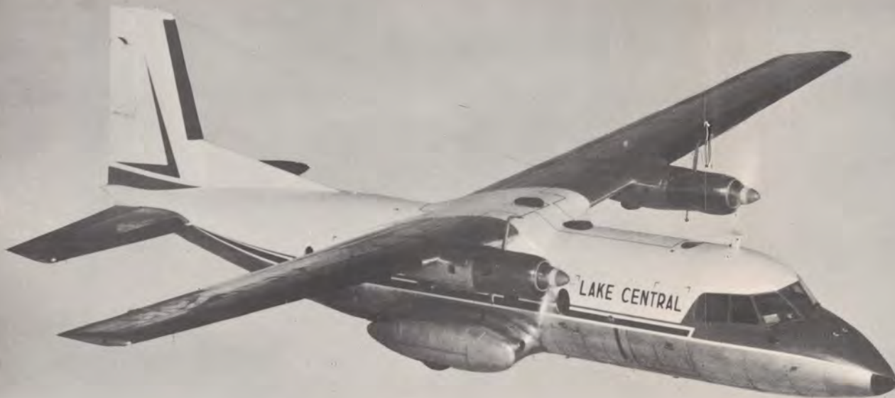
Nord 262 in flight. This French-built turbo-prop will become a familiar sight in U. S. sky this summer. A high-wing, 27-passenger, twin-engine aircraft, Lake Central Airlines has purchased a fleet of eight as initial replacements for their 24-passenger DC-3s. Plane cruises at 226 miles per hour as compared to DC-3's 170. Selection of the Nord climaxed a five-year search by the company to find a transport suitable for its short-haul, high-density routes. Right: Nord fuselage assembly area. Plane marked No. 9 is actually Lake Central's No. 1. Below: Air carrier specialists from FAA's Central Region at the Nord factory, from left: Marian (Bud) Shaw, Mordecai X. Crouse, Leonard Korenek, William R. Miller and Joseph Block. Above left: K. D. Mackenzie, chief of the Central Region's Air Carrier Branch (seated) and Mordecai X. Crouse admire a scale model of the new Nord 262.
