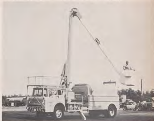
Charles P. Donovan, chief of automotive equipment, stands in the bucket of a multi-purpose electrical line maintenance bucket truck designed at NAFEC. It is a combination of the chassis and parts of many vehicles. The bucket is insulated to withstand 80,000 volts.
