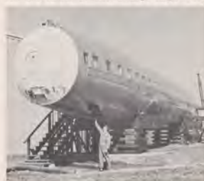
Aircraft fuselage used as laboratory to determine if protective standards are adequate for the detection and control of fires in large cargo areas.
