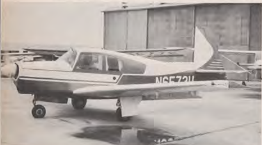
This Mooney Mark 21 is the most popular plane for long trips. Purchased in a damaged condition, it had only 100 hours flight time, so members restored it to new condition and added navigation equipment.
