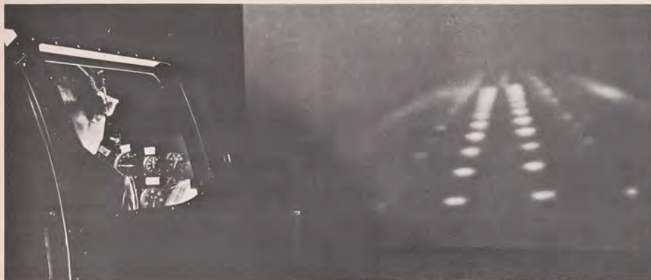
Above: This is how it looks to the pilot just a few moments before touchdown. In this environment a variety of landing aids under different ceiling and visibility combinations can be safely evaluated.
