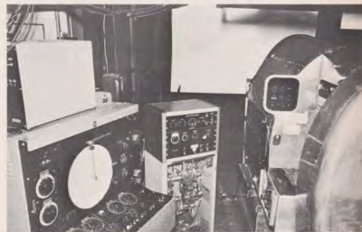
Above: A wider view of the P-3 flight simulator shows the projection screen in background. Below: Electronics technician Harry M. Halvorsen sets different flight conditions for the flight simulator pilot.
