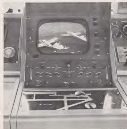
TV brings areas of restricted visibility into Salt Lake City control tower.
