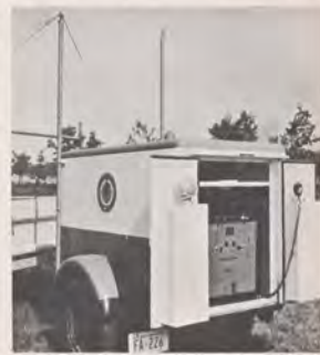
Ex-Navy communication trailer, restored by EA's SMS-105, has two receivers and one transmitter.
