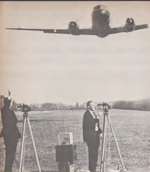
Above: Leonard Heaton (right) and German engineer make final check using radio theodolites. Below: approach to runway 27L crosses cemetery. Towering above the scene are light bars of approach light system. Final bars are on roofs of apartment buildings surrounding airport.
