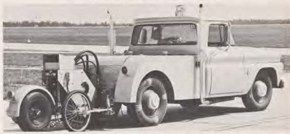
Newest addition to NAFEC's experimental equipment is a runway traction measuring vehicle developed for aircraft braking and skid research. It can reach speeds above 100 mph, accelerating from zero to 80 mph in 1,500 feet.
