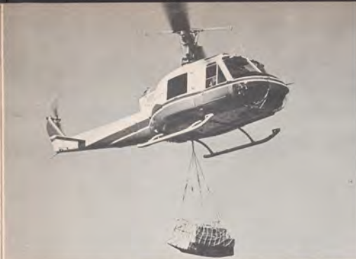
Supplies are moved quickly to remote area by helicopter using external slingload. 'Copter's accurate placement (right) of sections helps build tower in 30 minutes.
