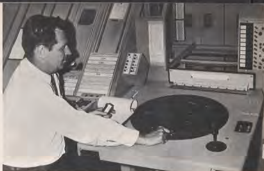
Electronic Maintenance Technician Lyle Adams working on RAPPI, newest computer/symbol generator that converts digital messages into suitable form for display on the radar screen. The signals are sent over ordinary phone lines.
