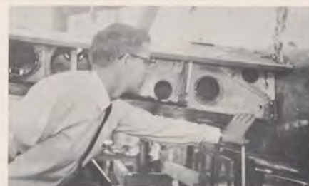
Stoner inspecting redesigned rear spar fitting after weakness showed up in testing. Below: wires leading to strain gauges are spotted throughout plane to measure effects.
