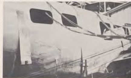
Stoner inspecting redesigned rear spar fitting after weakness showed up in testing. Below: wires leading to strain gauges are spotted throughout plane to measure effects.
