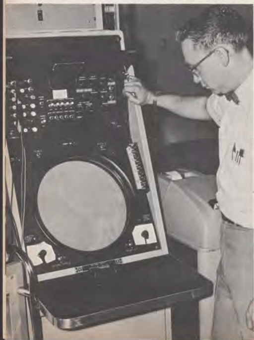
RAPPI gives air traffic control specialist increased radar information. William Waring of the Minneapolis Center observes the new RAPPI system.
