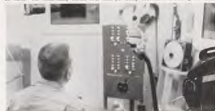
Upon rapid decompression (above), the chamber instantly fills with clouds of vapor. The pilot must don the oxygen mask and headphones before he can return to his tasks. The panel of lights (below) keeps the pilot alert to the problems at hand. He must keep hands and feet perfectly coordinated during the test.
