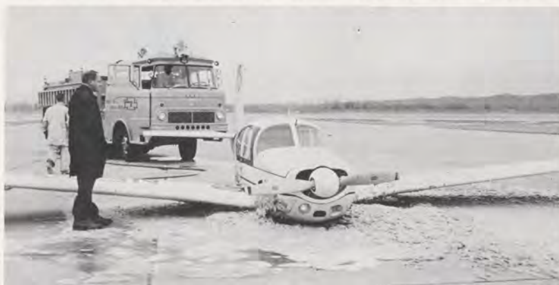
U.S. Air Force Major Roscoe E. Sprinkel checks over the wheels-up Mooney Mark 20. Seconds after the belly landing an Airport Authority crash vehicle quickly sprayed foam on the aircraft to minimize fire hazard.
