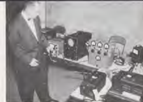
Using a strain-gaged aluminum beam Nauert demonstrates structural vibration of aircraft being tested.
