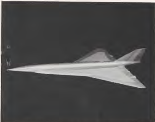
Lockheed's entry has double delta wing plan for development of Mach 3 plane.
