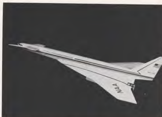
Canard wing aft of pilot compartment is unique feature of North American SST.
