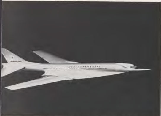
Boeing's 733 features variable sweep arrow wing that can be moved in flight.
