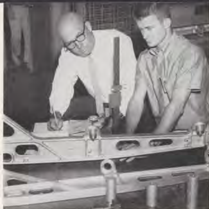
Dale A. Miller (l.), manufacturing inspector of EMDO-41, gives a detail inspection to a critical forging to determine that it conforms with the approved design. The part is also checked to determine if previous plant inspections followed FAA approved quality control procedures for the aircraft.
