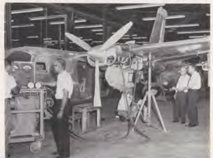
A final functional check of the aircraft landing gear retraction system is being made by inspectors. All systems are checked out before flight testing.
